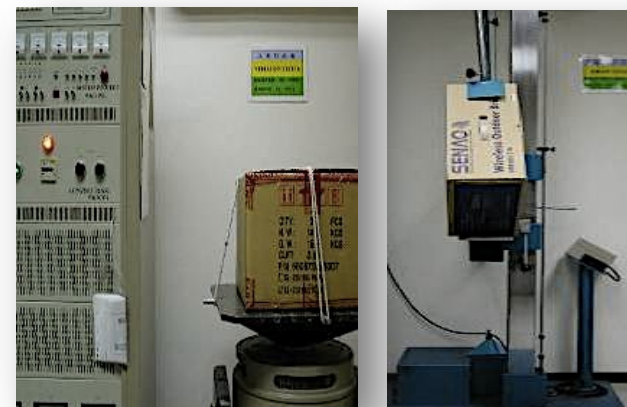
Vibration &amp; Drop Test
